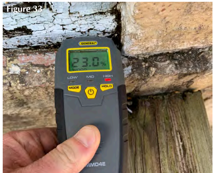
Several locations with high moisture content at sills
